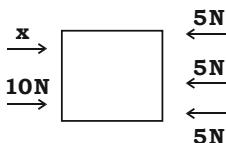
**Sol.** A/Q Balanced force, So  $R_f = 0$
